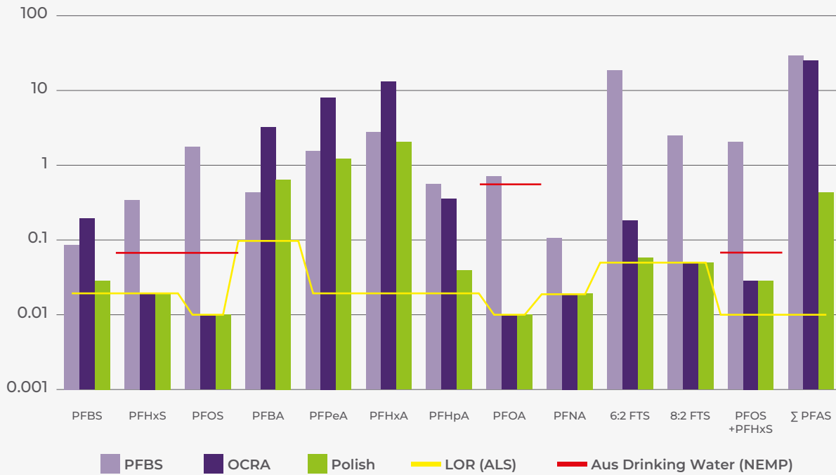
Reduction in PFAS Concentration via OCRA and then NF/RO (TOP Assay PFAS Analysis) Log Scale Plot
